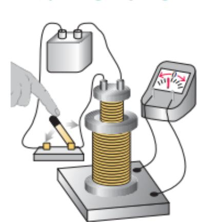
\*They cause the magnetic field through the coil to *change*.
